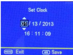
Press the ▲ ▼ button to set the **MONTH**, then press the ► button to navigate to the **DATE** and use the ▼ ▲ buttons to set the date. Press the ► button to navigate to the year and set that using the ▲ ▼ buttons.
