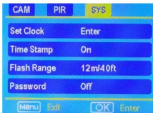
**SETTING THE CLOCK:** Scroll over to the **SYS** tab using the ► ◀ buttons and then press the ▼ button to highlight the **Set Clock** option. Press **OK**. You will see the following screen. (Fig 11)
